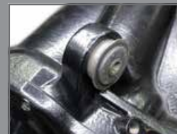
INTEGRATED UPPER CONTROL ARM MOUNT
