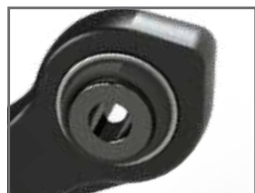
RUBBER BUSHING FOR REDUCED NVH
