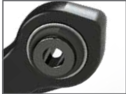
RUBBER BUSHING FOR REDUCED NVH
