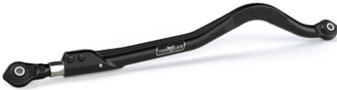
RUBBER BUSHING FOR REDUCED NVH
