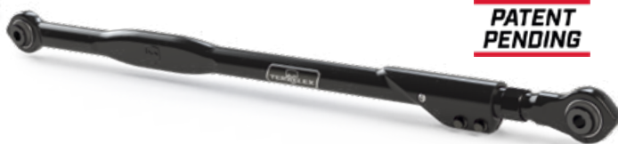
RUBBER BUSHING FOR REDUCED NVH
